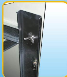
11. Tight 16 sets M6 screws, washes and nuts for 4 door plates
